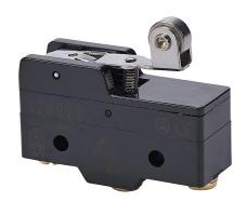
IDEM micro limit switch, lever hinge with steel roller, (1) N.O./(1) N.C. contact(s), snap action, 25.4mm hole spacing, polybutylene terephthalate, screw terminals.
