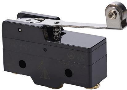
IDEM micro limit switch, lever hinge long with steel roller, (1) N.O./ (1) N.C. contact(s), snap action, 25.4mm hole spacing, polybutylene terephthalate, screw terminals. Package of 5.
