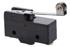
IDEM micro limit switch, lever hinge long with steel roller, (1) N.O./ (1) N.C. contact(s), snap action, 25.4mm hole spacing, polybutylene terephthalate, screw terminals. Package of 5.
