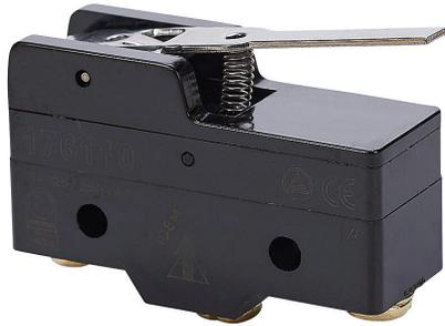
IDEM micro limit switch, lever hinge, (1) N.O./ (1) N.C. contact(s), snap action, 25.4mm hole spacing, polybutylene terephthalate, screw terminals. Package of 5.
