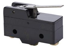
IDEM micro limit switch, lever hinge, (1) N.O./(1) N.C. contact(s), snap action, 25.4mm hole spacing, polybutylene terephthalate, screw terminals. Package of 5.
