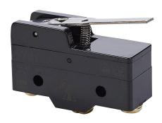
IDEM micro limit switch, lever hinge, (1) N.O./(1) N.C. contact(s), snap action, 25.4mm hole spacing, polybutylene terephthalate, screw terminals.
