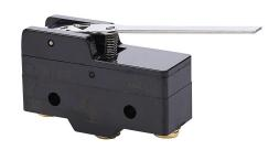
IDEM micro limit switch, lever hinge long, (1) N.O./(1) N.C. contact(s), snap action, 25.4mm hole spacing, polybutylene terephthalate, screw terminals.
