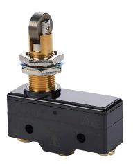
IDEM micro limit switch, metal plunger with metal cross roller and fixing nuts, (1) N.O./(1) N.C. contact(s), snap action, 25.4mm hole spacing, polybutylene terephthalate, screw terminals. Package of 5.
