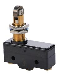
IDEM micro limit switch, metal plunger with metal cross roller and fixing nuts, (1) N.O./(1) N.C. contact(s), snap action, 25.4mm hole spacing, polybutylene terephthalate, screw terminals.
