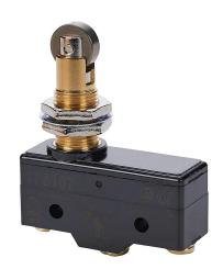
IDEM micro limit switch, metal plunger with metal roller and fixing nuts, (1) N.O./(1) N.C. contact(s), snap action, 25.4mm hole spacing, polybutylene terephthalate, screw terminals. Package of 5.
