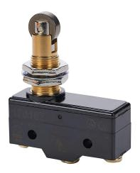
IDEM micro limit switch, metal plunger with metal roller and fixing nuts, (1) N.O./(1) N.C. contact(s), snap action, 25.4mm hole spacing, polybutylene terephthalate, screw terminals.
