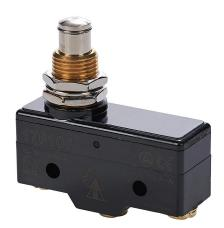
IDEM micro limit switch, metal plunger with fixing nuts, (1) N.O./ (1) N.C. contact(s), snap action, 25.4mm hole spacing, polybutylene terephthalate, screw terminals. Package of 5.
