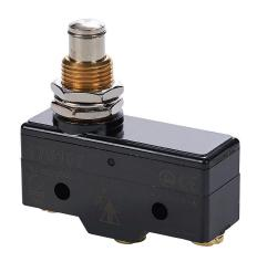
IDEM micro limit switch, metal plunger with fixing nuts, (1) N.O./ (1) N.C. contact(s), snap action, 25.4mm hole spacing, polybutylene terephthalate, screw terminals.
