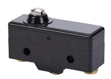
IDEM micro limit switch, metal plunger, (1) N.O./(1) N.C. contact(s), snap action, 25.4mm hole spacing, polybutylene terephthalate, screw terminals.
