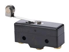
IDEM micro limit switch, lever with steel roller, (1) N.O./(1) N.C. contact(s), snap action, 25.4mm hole spacing, polybutylene terephthalate, screw terminals. Package of 5.
