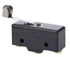
IDEM micro limit switch, lever with steel roller, (1) N.O./(1) N.C. contact(s), snap action, 25.4mm hole spacing, polybutylene terephthalate, screw terminals.
