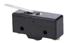
IDEM micro limit switch, lever, (1) N.O./(1) N.C. contact(s), snap action, 25.4mm hole spacing, polybutylene terephthalate, screw terminals. Package of 5.
