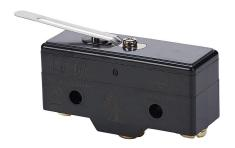
IDEM micro limit switch, lever, (1) N.O./(1) N.C. contact(s), snap action, 25.4mm hole spacing, polybutylene terephthalate, screw terminals.
