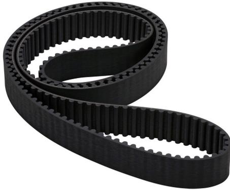
SureMotion timing belt, 8mm 8M pitch, 30mm wide, 220 tooth, 1760mm pitch length (circumference), neoprene, fiberglass reinforced.
