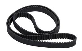
SureMotion timing belt, 8mm 8M pitch, 20mm wide, 220 tooth, 1760mm pitch length (circumference), neoprene, fiberglass reinforced.
