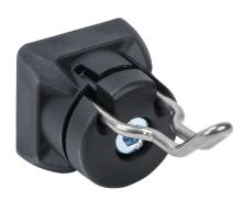
FATH tool hook, black, 24/16 - 12, glass ball reinforced nylon/stainless steel/steel, slot size 8/10. For use with all 1.5in, 3in, 40mm, 45mm, 80mm and 90mm profile T-slotted rails. Manufacturer part number: 6TH240NA5020S01.
