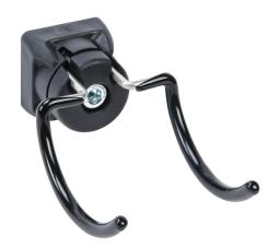
FATH tool double hook, black, R35 - 67, glass ball reinforced nylon/stainless steel/steel, slot size 8/10. For use with all 1.5in, 3in, 40mm, 45mm, 80mm and 90mm profile T-slotted rails. Manufacturer part number: 6TH240NR3091S01.
