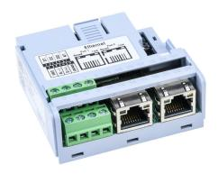
WEG Electric CFW500 series communication module, EtherNet/IP, Modbus TCP, Modbus RTU, BACnet and webserver, 3 ports, (2) Ethernet (RJ45) and (1) RS-485 (3-pin terminal) port(s). For use with WEG CFW500 series AC drives.
