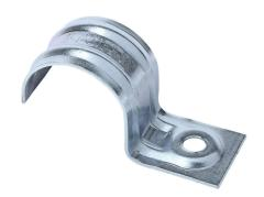
Minerallac 1-hole conduit mount strap, standard duty. Package of 100. For use with 1-1/4in RMC/IMC/LFMC, 1-1/2in EMT, 1-1/2in FMC.
