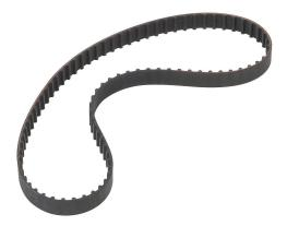
SureMotion timing belt, 1/5in XL pitch, 3/8in wide, 85 tooth, 17in pitch length (circumference), neoprene, fiberglass reinforced.
