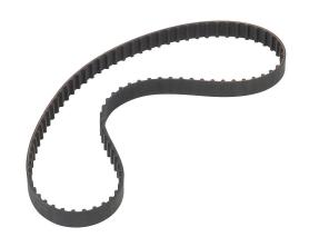
SureMotion timing belt, 1/5in XL pitch, 3/8in wide, 85 tooth, 17in pitch length (circumference), neoprene, fiberglass reinforced.
