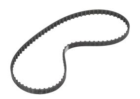
SureMotion timing belt, 1/5in XL pitch, 1/4in wide, 85 tooth, 17in pitch length (circumference), neoprene, fiberglass reinforced.
