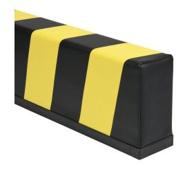
ASO Safety Solutions safety contact bumper, 100 x 200mm, 5ft length, (1) 3-pin male M8 connector and (1) 3-pin female M8 connector, 4.7in/120mm cable length. Aluminum mounting rail included.
