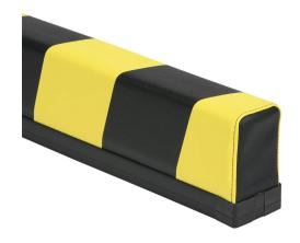
ASO Safety Solutions safety contact bumper, 60 x 100mm, 5ft length, (1) 3-pin male M8 connector and (1) 3-pin female M8 connector, 4.7in/120mm cable length. Aluminum mounting rail included.
