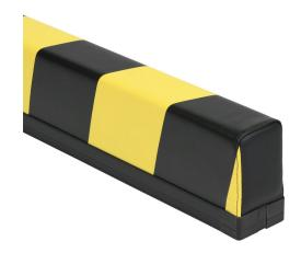
ASO Safety Solutions safety contact bumper, 60 x 100mm, 4ft length, (1) 3-pin male M8 connector and (1) 3-pin female M8 connector, 4.7in/120mm cable length. Aluminum mounting rail included.
