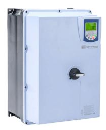
WEG Electric CFW500 series AC high-performance drive with disconnect, NEMA 4X, 460 VAC, 30hp with 3-phase input, SVC, V/Hz, VVW, FOC, encoder or torque mode, C frame, RS-485, integrated dynamic braking. Optional communication and STO modules available.
