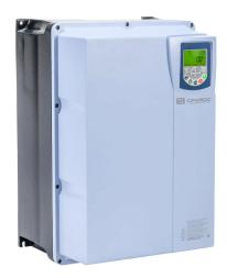
WEG Electric CFW500 series AC high-performance drive, NEMA 4X, 230 VAC, 15hp with 3-phase input, SVC, V/Hz, VVW, FOC, encoder or torque mode, C frame, RS-485, integrated dynamic braking. Optional communication and STO modules available.
