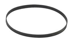
SureMotion timing belt, 0.08in MXL pitch, 1/4in wide, 166 tooth, 13.3in pitch length (circumference), neoprene, fiberglass reinforced. Package of 3.
