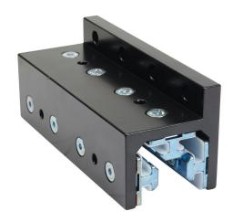
FATH 3-slot single-flange linear bearing, black, 63 x 160 x 67mm, aluminum/die-cast zinc/polyoxymethylene (POM), slot size 8. For use with all 40mm profile T-slotted rails. Manufacturer part number: 093SF402S.
