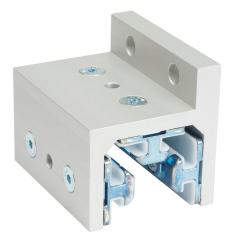
FATH 3-slot single-flange linear bearing, silver, 63 x 80 x 67mm, aluminum/die-cast zinc/polyoxymethylene (POM), slot size 8. For use with all 40mm profile T-slotted rails. Manufacturer part number: 093SF401.
