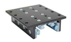
FATH 4-slot double-flange linear bearing, black, 143 x 160 x 48mm, aluminum/die-cast zinc/polyoxymethylene (POM), slot size 8. For use with all 80mm profile T-slotted rails. Manufacturer part number: 093DF802S.
