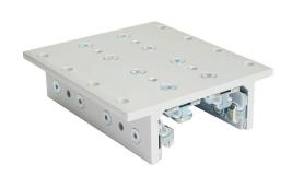
FATH 4-slot double-flange linear bearing, silver, 143 x 160 x 48mm, aluminum/die-cast zinc/polyoxymethylene (POM), slot size 8. For use with all 80mm profile T-slotted rails. Manufacturer part number: 093DF802.
