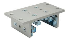
FATH 4-slot double-flange linear bearing, silver, 143 x 80 x 48mm, aluminum/die-cast zinc/polyoxymethylene (POM), slot size 8. For use with all 80mm profile T-slotted rails. Manufacturer part number: 093DF801.
