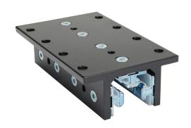
FATH 3-slot double-flange linear bearing, black, 103 x 160 x 48mm, aluminum/die-cast zinc/polyoxymethylene (POM), slot size 8. For use with all 40mm profile T-slotted rails. Manufacturer part number: 093DF402S.
