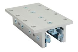
FATH 3-slot double-flange linear bearing, silver, 103 x 160 x 48mm, aluminum/die-cast zinc/polyoxymethylene (POM), slot size 8. For use with all 40mm profile T-slotted rails. Manufacturer part number: 093DF402.
