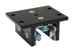
FATH 3-slot double-flange linear bearing, black, 103 x 80 x 48mm, aluminum/die-cast zinc/polyoxymethylene (POM), slot size 8. For use with all 40mm profile T-slotted rails. Manufacturer part number: 093DF401S.
