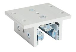
FATH 3-slot double-flange linear bearing, silver, 103 x 80 x 48mm, aluminum/die-cast zinc/polyoxymethylene (POM), slot size 8. For use with all 40mm profile T-slotted rails. Manufacturer part number: 093DF401.
