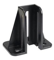
FATH foot console, black, 40 x 40mm, die-cast aluminum, slot size 8. For use with all 40mm T-slotted rails. Manufacturer part number: 098G38L85128AS.
