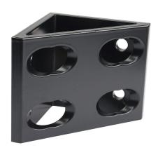
FATH gusseted inside corner bracket, black, 90-degree, 8 holes, aluminum, slot size 8. For use with all 40mm and 80mm profile T-slotted rails. Manufacturer part number: 093W8806N08S.
