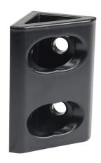
FATH wide gusseted inside corner bracket, black, 90-degree, 4 holes, aluminum, slot size 8. For use with all 40mm and 80mm profile T-slotted rails. Manufacturer part number: 093WD8404N08S.
