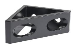
FATH tall gusseted inside corner bracket, black, 90-degree, 4 holes, aluminum, slot size 8. For use with all 40mm and 80mm profile T-slotted rails. Manufacturer part number: 093W8403N08S.
