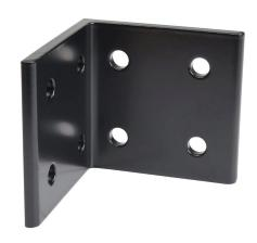
FATH inside corner bracket, black, 90-degree, 8 holes, aluminum, slot size 8. For use with all 40mm and 80mm profile T-slotted rails. Manufacturer part number: 093WD8080S.
