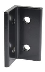
FATH wide inside corner bracket, black, 90-degree, 4 holes, aluminum, slot size 8. For use with all 40mm and 80mm profile T-slotted rails. Manufacturer part number: 093WD8040S.
