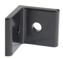
FATH inside corner bracket, black, 90-degree, 2 holes, aluminum, slot size 8. For use with all 40mm and 80mm profile T-slotted rails. Manufacturer part number: 093WD40S.
