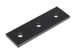
FATH straight flat plate, black, 3 holes, aluminum, slot size 8. For use with all 40mm and 80mm profile T-slotted rails. Manufacturer part number: 093VA40120S.
