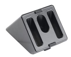
FATH angle connector, black, 45-degree, 40 x 40mm, die-cast aluminum, slot size 8. For use with all 40mm and 80mm profile T-slotted rails. Manufacturer part number: 093WS40145N08S.
