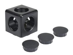
FATH 3D cube connector, black, 40 x 40 x 40mm, die-cast aluminum, slot size 8. For use with all 40mm and 80mm profile T-slotted rails. (3) plastic cover caps included. Manufacturer part number: 093WW406N0S.
