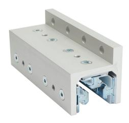
FATH 3-slot single-flange linear bearing, silver, 63 x 160 x 67mm, aluminum/die-cast zinc/polyoxymethylene (POM), slot size 8. For use with all 1.5in profile T-slotted rails. Manufacturer part number: 093SF382.
